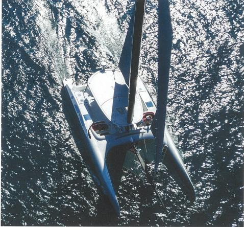
modulus fibres but rarely metal – in the construction of the Eagle. Born in a shop that specialises in high-end composites, critical components in the Eagle Class 53 are carbon prepreg formed in female moulds and then baked and autoclaved.
